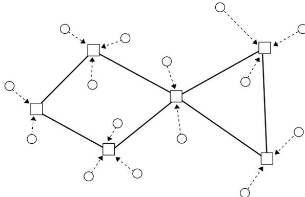
Figure 1: *An example of 2-edge connected/star network*
